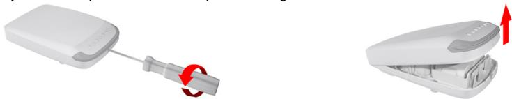
Figure 2: Removing the Top Cover
