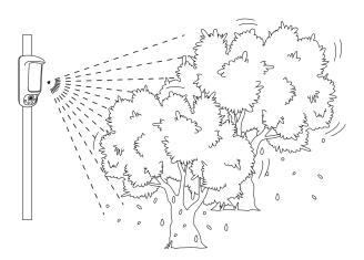
In order to maximize detection efficiency, choose a location that is most likely to intercept intruders moving across the coverage area at a 45 degree angle.
