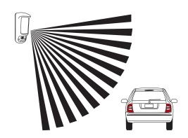
Avoid installing the detector near moving objects (e.g., swaying trees, bushes, etc.).
