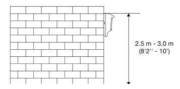
If the installation site is near heavy traffic or objects beyond the required detection range, adjust the MW sensitivity and/or tilt the detector down.
