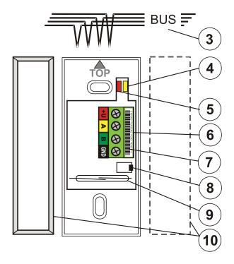
Fig: 3 – bus cable; 4 – yellow fault indicator; 5 – red detector activation indicator; 6 – digital bus terminals; 7 – production code; 8 – tamper contact; 9 – magnetic sensor; 10 – permanent magnet with its alternative position
