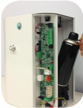
Fast 03 1C is the ideal fogging system to protect small /medium areas like shops, homes, bank ATM machines. It is the entry level of the professional line, shoots up to 200/300 m3 of dense fog in about 20 seconds. It is equipped with a single cylinder and the shooting may be set in seconds. It is very fast and competitive.
