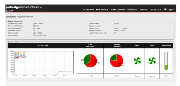
A comprehensive GUI enables incredible control over the powerful features of the S3 Switch. Firmware updates, management, security features, and enhanced configurations are available at the click of a button. Useful diagnostics are displayed directly on the dashboard, including fan speeds, temperatures, and both RAM and CPU utilization.
