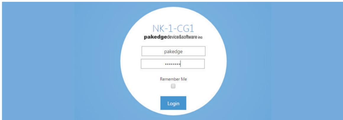
**NOTE:** If your computer is not set to the default IP scheme of the NK-1 (192.168.1.X), you must first configure the TCP/IP settings on your computer to log in to the NK-1 through a web browser.
