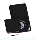
Re-install the battery with the positive (+) side facing up. Slide the Keyfob battery cover closed.
