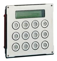
Module made using double 2.5 mm 316 stainless steel plate, complete with keypad featuring 12 backlit buttons and 16-digit alphanumeric display showing call codes and user interaction messages (busy, etc.). Also functions as an electronic key code with 1000 possible different 6-digit command codes. Dimensions: 106x106x56 mm. Compatible only with the art. 4680, 4680C, 4681, 4682HC, 4682HD, 1621, 1621VC, 1622, 1622VC, 1682 and 1682HVC combined with the fronts art. 3262S/x and 3268S/x.
