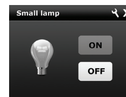
Fig.3 Icon of Fibaro Switch shown by Home Center controller
