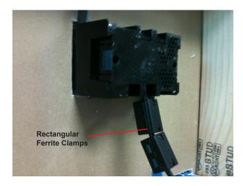
Ferrite Clamp Installation when Using AC Power and a WiFi Network Connection
