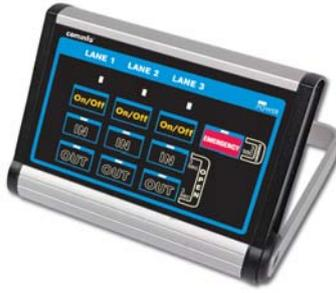
**TOUCH::PANEL** - Touch-button panel for remote control of turnstiles and gates
