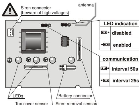
**LED ON / OFF** enables short flashes of the siren every 60 seconds (= position ON). If OFF is selected, the siren will flash only while indicating an alarm.
