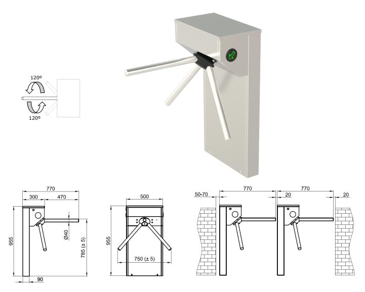
**Power Requirements** : 110/220V. 60/50Hz. AC (%±10) 24V. DC at standby ~11W. max. ~60W.
