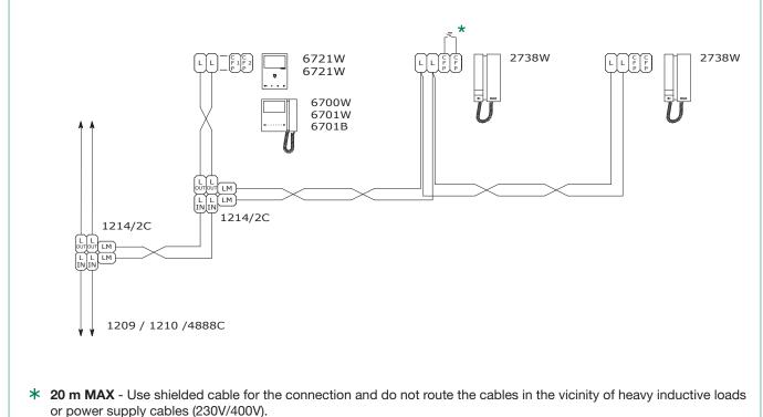
Where multiple door-entry phones or monitor backplates have the same user code, connect the CFP button on one only; all the devices will ring simultaneously.
