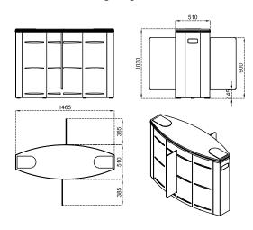
SG 90 M-S Glass Wing Height: 1200 mm
